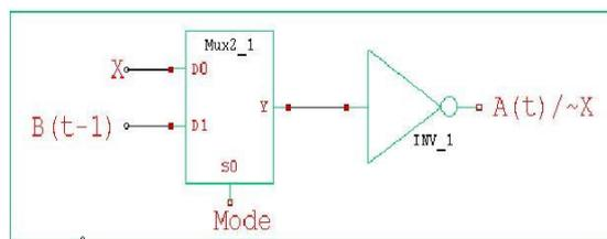
Fig. 9. Sharing of Logic Operation for A(t) and X
