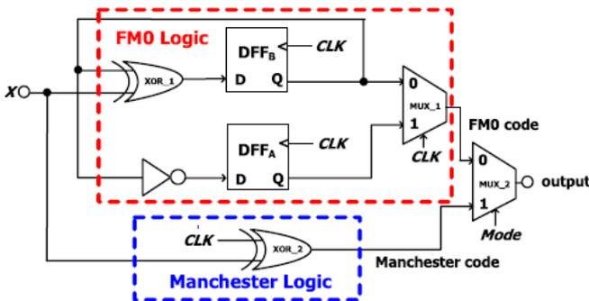
Fig. 6. VLSI Hardware architecture of FMO, Manchester encodings.
