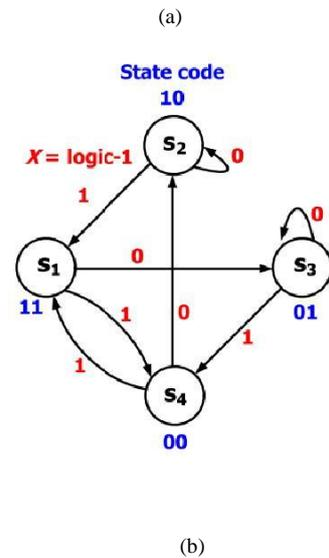
Fig. 5. FSM for FMO. (a) Definition of states (b) FSM of FMO
