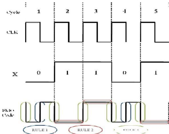
Fig. 3. Example of FMO coding
