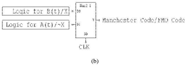
Fig. 8. Working of Sharing of Logic Operation (a) Manchester encodings in Multiplexer. (b) Combination of FMO and Manchester encodings
