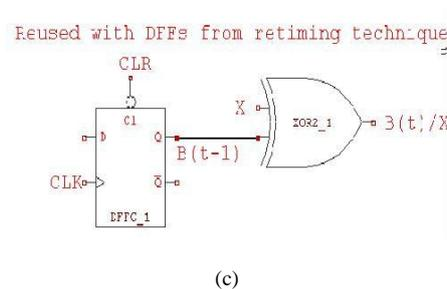
Fig. 10. Logic operation Sharing of B(t), X. (a) Without XOR sharing. (b) With XOR sharing. (c) Reused DFF1
