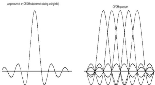
Figure: 3 OFDM Spectrum
