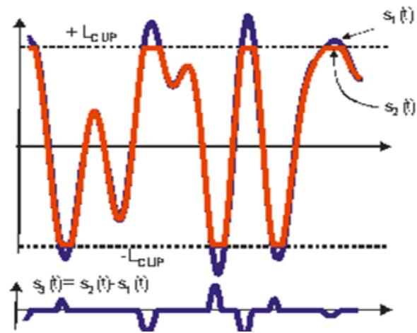
Figure: 4 Clipping and Filtering of Signal
