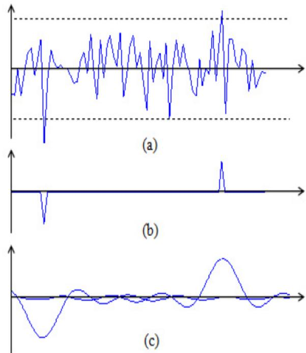
Figure: 10 Peak Cancellation (a) OFDM signal (b) Identified peak (c) scaled and shifted peak cancellation waveform
