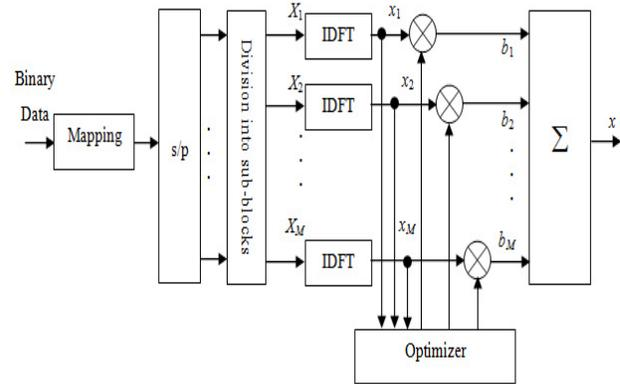
Figure: 13 Block diagram of OFDM transmitter with PTS
