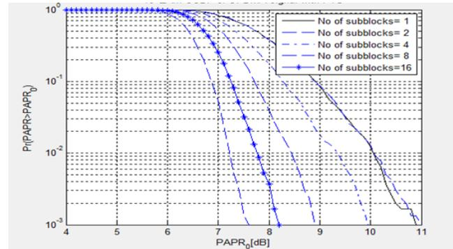
Figure: 14 QAM CCDF of OFDM signal with PTS
