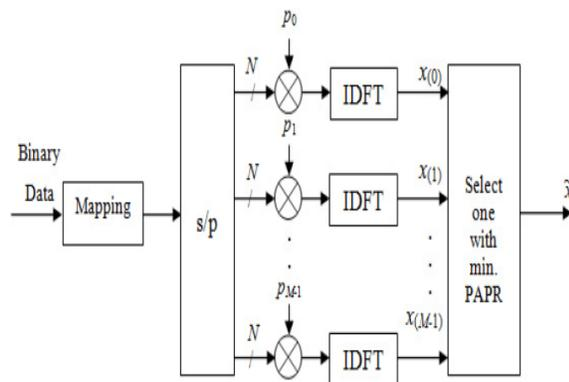
Figure: 9 Block diagram of OFDM transmitter with SLM
