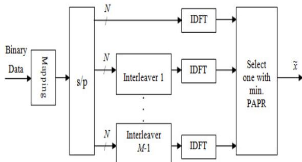
Figure: 15 Block diagram of Interleaved OFDM transmitter
