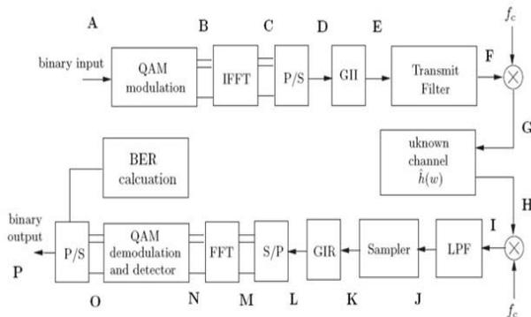
Figure: 1 OFDM Transmitter and Receiver
