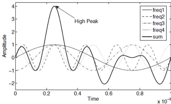
Figure: 2 High peaks in OFDM signal generated by summing multiple sinusoids
