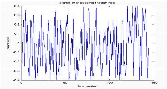
Figure: 7 signal after PAPR reduction (Clipped signal)
