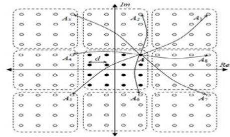
Figure: 16 Tone injection technique for 16-QAM constellation
